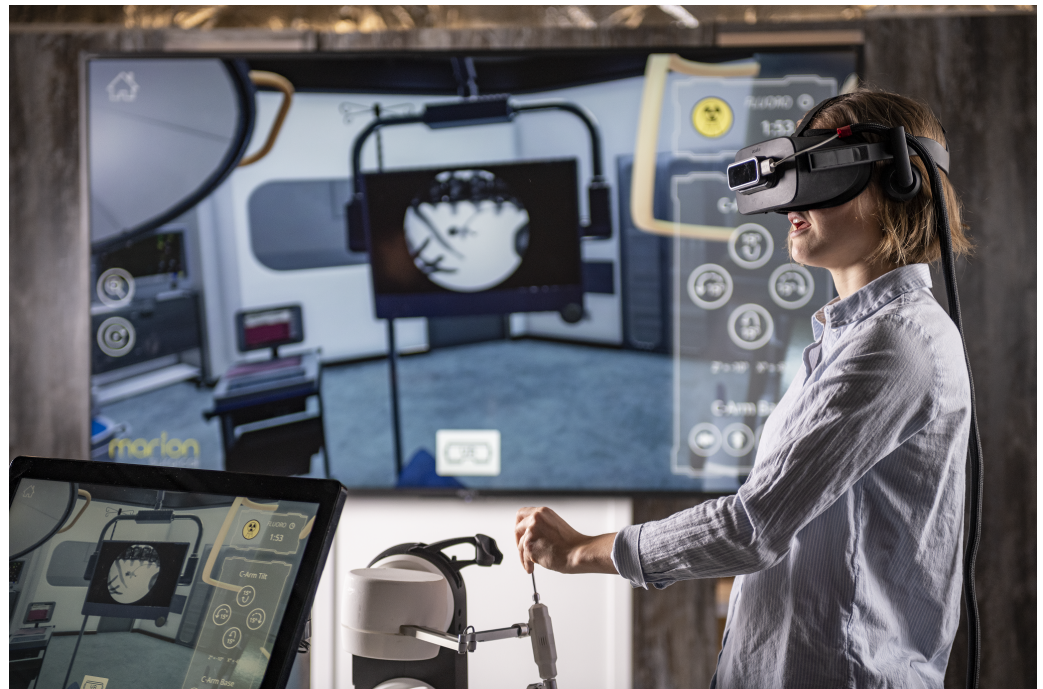
Figure 2. The virtual operating room of the Marion K181 PCNL simulator is shown with a user operating the haptic device, a virtual patient undergoing PCNL, virtual X-ray imaging, and the medical instruments and imaging device, which would be present in the real world operating room. The user is wearing a VR headset with the leap motion attachment for hand tracking. The TV screen behind the user shows a representation of what the user sees in VR, the X-ray view and the Virtual Reality Operating room. The user's hands are holding the needle tool that is attached to the haptic robots that provide real-time force feedback.
